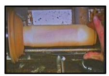
For the stem a length of Yew branch was mounted between centres and roughed to round, a parting tool was used to form a spigot to fit into the hole in the base. The chuck and base were refitted onto the lathe and the column inserted. A small tenon was formed at
